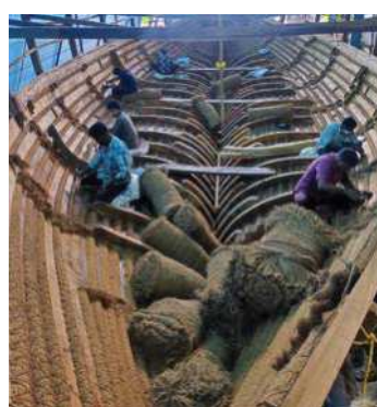
The 21 metre stitched ship undergoing construction at the Hodi Innovations shipyard in Divar Island
