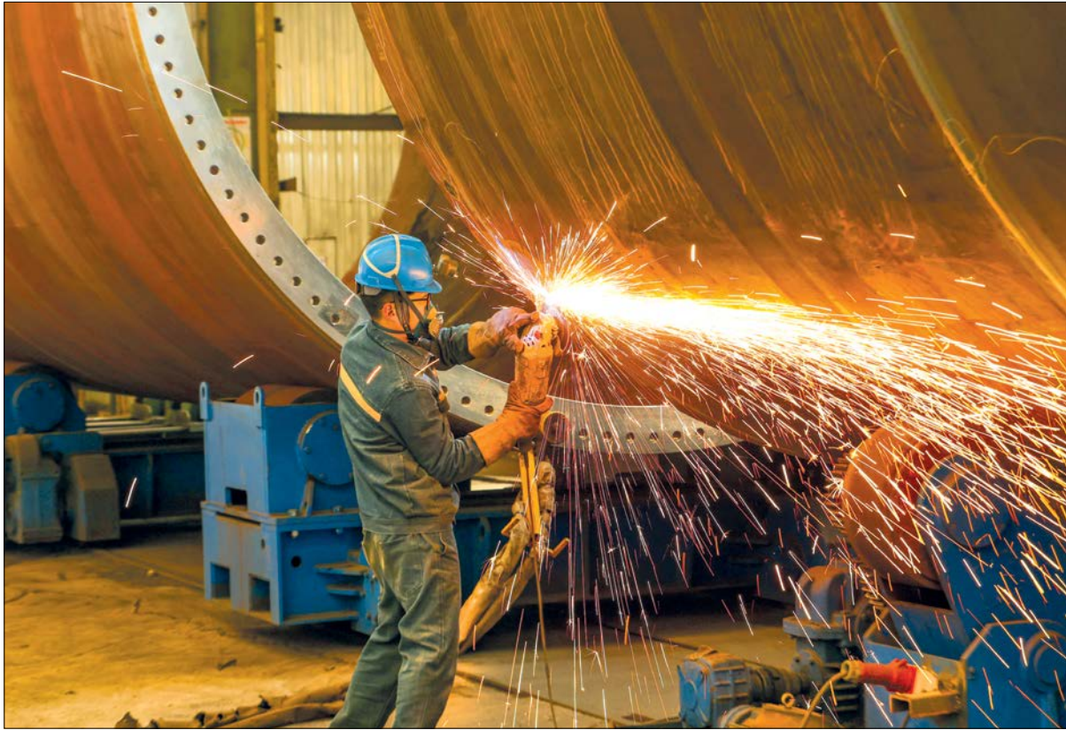
A worker grinds a section of the tower of a wind turbine in the workshop of a wind power equipment company in Lianyungang, in China's eastern Jiangsu province, on Wednesday
